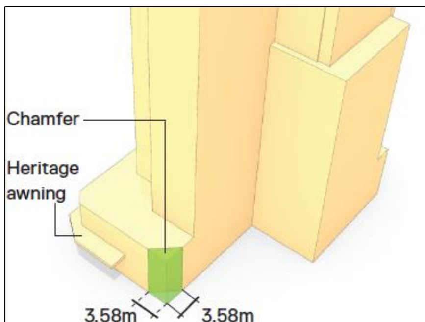
Figure 1: Podium Chamfer (Source: Grimshaw)
